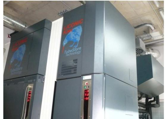
**Combined manual and fully automated system of  $-80^{\circ}\text{C}$**
